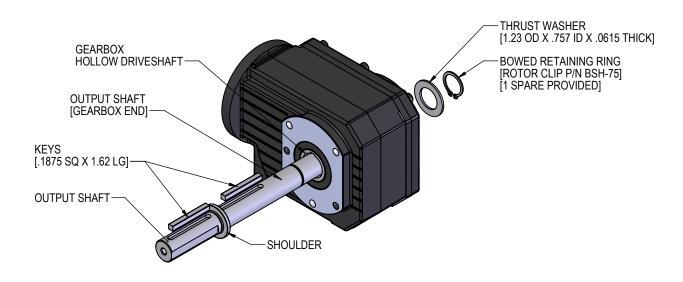
1. Insert key into keyway on gearbox end of output shaft.
