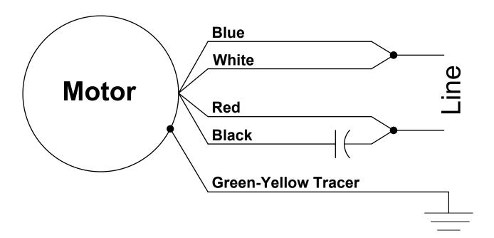
Direction of Rotation: Clockwise To reverse direction of rotation, transpose Blue & Red leads.
