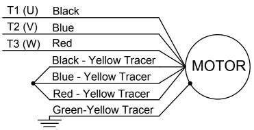
**Direction of Rotation: Clockwise** To reverse direction of rotation. transpose any two line leads.
