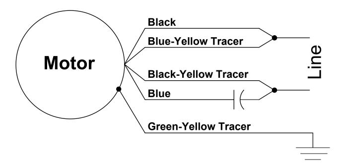
**Direction of Rotation: Clockwise**To reverse direction of rotation,
