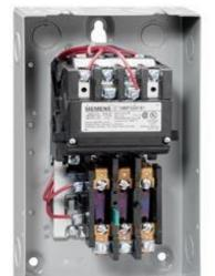
Non-reversing motor starter Size 00 Three phase full voltage Amb compensate bimetal OLrelay Contactor amp rating 9Amp Non-combination type Enclosure NEMA type 1 Indoor general purpose use Standard width enclosure
