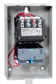
Non-reversing motor starter Size 00 Three phase full voltage Solidstate overload relay OLRelay amp range 0.25-1A 24Vdc coil Noncombination type Enclosure NEMA type 1 Indoor general purpose use Standard width enclosure
