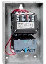
Non-reversing motor starter Size 00 Three phase full voltage Solidstate overload relay OLRelay amp range 0.75-3.4A 24Vdc coil Noncombination type Enclosure NEMA type 1 Indoor general purpose use Extra-wide enclosure
