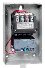
Non-reversing motor starter Size 00 Three phase full voltage Solidstate overload relay OLRelay amp range 3-12A 24Vdc coil Noncombination type Enclosure NEMA type 1 Indoor general purpose use Extra-wide enclosure
