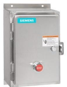
Non-reversing motor starter Size 1 Three phase full voltage Solidstate overload relay OLRelay amp range 0.25-1A 24Vdc coil Noncombination type Encl NEMA type 4X 304 S-steel Water/dust tight non-corrosive Extra-wide enclosure
