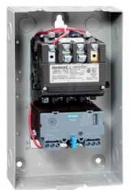
Non-reversing motor starter Size 1 Three phase full voltage Solidstate overload relay OLRelay amp range 0.75-3.4A 24Vdc coil Noncombination type Enclosure NEMA type 1 Indoor general purpose use Standard width enclosure
