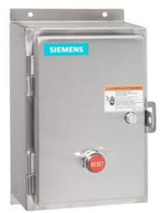
Non-reversing motor starter Size 1 Three phase full voltage Solidstate overload relay OLRelay amp range 0.75-3.4A 24Vdc coil Noncombination type Encl NEMA type 4X 304 S-steel Water/dust tight non-corrosive Extra-wide enclosure
