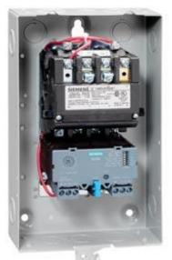
Non-reversing motor starter Size 1 Three phase full voltage Solidstate overload relay OLRelay amp range 3-12A 208VAC 60HZ coil Non-combination type Enclosure NEMA type 1 Indoor general purpose use Extra-wide enclosure
