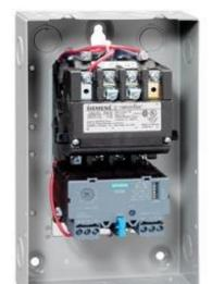
Non-reversing motor starter Size 1 Three phase full voltage Solidstate overload relay OLRelay amp range 3-12A 24Vdc coil Noncombination type Enclosure NEMA type 1 Indoor general purpose use Extra-wide enclosure
