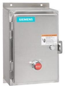
Non-reversing motor starter Size 1 Single phase full voltage Solidstate overload relay OLRelay amp range 5.5-22A 110VAC 50HZ / 120VAC 60HZ coil Non-combination type Encl NEMA type 4X 316 Ssteel Water/dust tight non-corrosive Standard width enclosure
