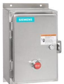
Non-reversing motor starter Size 1 Single phase full voltage Solidstate overload relay OLRelay amp range 5.5-22A Non-combination type Encl NEMA type 4X 316 S-steel Water/dust tight non-corrosive Standard width enclosure
