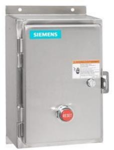
Non-reversing motor starter Size 1 Single phase full voltage Solidstate overload relay OLRelay amp range 5.5-22A 24VAC 50-60HZ coil Non-combination type Encl NEMA type 4X 316 S-steel Water/dust tight non-corrosive Standard width enclosure
