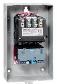
Non-reversing motor starter Size 1 Three phase full voltage Solidstate overload relay OLRelay amp range 5.5-22A 24Vdc coil Noncombination type Enclosure NEMA type 1 Indoor general purpose use Extra-wide enclosure
