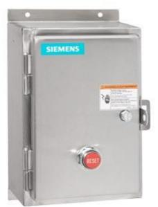
Non-reversing motor starter Size 1 Three phase full voltage Solidstate overload relay OLRelay amp range 5.5-22A 24Vdc coil Noncombination type Encl NEMA type 4X 304 S-steel Water/dust tight non-corrosive Extra-wide enclosure
