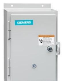
Non-reversing motor starter Size 1 Three phase full voltage Solidstate overload relay OLRelay amp range 10-40a 24Vdc coil Noncombination type Enclosure NEMA type 12 Dust/drip proof for indoors Extra-wide enclosure
