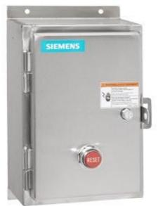
Non-reversing motor starter Size 1 3/4 Single phase, 2-pole Amb compensate bimetal OLrelay Contactor amp rating 40Amp 24VAC 50-60HZ coil Non-combination type Encl NEMA type 4X 316 S-steel Water/dust tight non-corrosive Standard width enclosure
