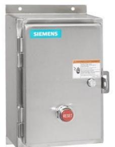
Non-reversing motor starter Size 2 Single phase, 2-pole Amb compensate bimetal OLrelay Contactor amp rating 45Amp 208VAC 60HZ coil Non-combination type Encl NEMA type 4X 304 S-steel Water/dust tight non-corrosive Standard width enclosure
