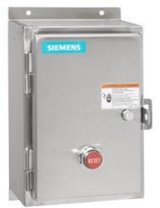
Non-reversing motor starter Size 2 Single phase, 2-pole Amb compensate bimetal OLrelay Contactor amp rating 45Amp 24VAC 50-60HZ coil Non-combination type Encl NEMA type 4X 304 S-steel Water/dust tight non-corrosive Standard width enclosure
