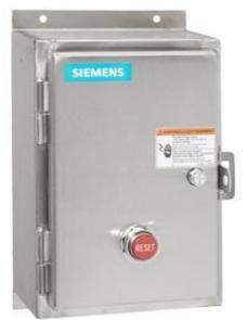
Non-reversing motor starter Size 2 Single phase, 2-pole Amb compensate bimetal OLrelay Contactor amp rating 45Amp 208VAC 60HZ coil Non-combination type Encl NEMA type 4X 316 S-steel Water/dust tight non-corrosive Standard width enclosure
