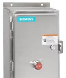
Non-reversing motor starter Size 2 Single phase, 2-pole Amb compensate bimetal OLrelay Contactor amp rating 45Amp 110VAC 50HZ / 120VAC 60HZ coil Non-combination type Encl NEMA type 4X 316 S-steel Water/dust tight non-corrosive Standard width enclosure
