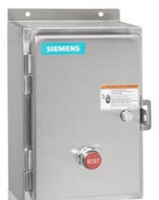
Non-reversing motor starter Size 2 Single phase, 2-pole Amb compensate bimetal OLrelay Contactor amp rating 45Amp Non-combination type Encl NEMA type 4X 316 S-steel Water/dust tight non-corrosive Standard width enclosure
