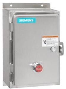
Non-reversing motor starter Size 2 Single phase, 2-pole Amb compensate bimetal OLrelay Contactor amp rating 45Amp 24VAC 50-60HZ coil Non-combination type Encl NEMA type 4X 316 S-steel Water/dust tight non-corrosive Standard width enclosure
