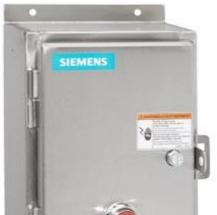
Non-reversing motor starter Size 2 Single phase, 2-pole Amb compensate bimetal OLrelay Contactor amp rating 45Amp 24Vdc coil Non-combination type Encl NEMA type 4X 316 S-steel Water/dust tight non-corrosive Standard width enclosure
