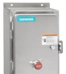
Non-reversing motor starter Size 2 Three phase full voltage Amb compensate bimetal OLrelay Contactor amp rating 45Amp Non-combination type Encl NEMA type 4X 304 S-steel Water/dust tight non-corrosive Standard width enclosure
