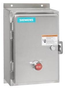
Non-reversing motor starter Size 2 Three phase full voltage Amb compensate bimetal OLrelay Contactor amp rating 45Amp 24VAC 50-60HZ coil Non-combination type Encl NEMA type 4X 304 S-steel Water/dust tight non-corrosive Standard width enclosure
