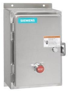
Non-reversing motor starter Size 2 Three phase full voltage Amb compensate bimetal OLrelay Contactor amp rating 45Amp 208VAC 60HZ coil Non-combination type Encl NEMA type 4X 316 S-steel Water/dust tight non-corrosive Standard width enclosure
