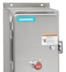
Non-reversing motor starter Size 2 Three phase full voltage Amb compensate bimetal OLrelay Contactor amp rating 45Amp Non-combination type Encl NEMA type 4X 316 S-steel Water/dust tight non-corrosive Standard width enclosure
