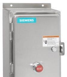
Non-reversing motor starter Size 2 Three phase full voltage Amb compensate bimetal OLrelay Contactor amp rating 45Amp 240VAC 50HZ / 277VAC 60HZ coil Non-combination type Encl NEMA type 4X 316 S-steel Water/dust tight non-corrosive Standard width enclosure
