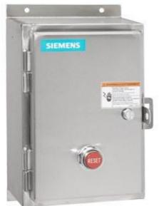
Non-reversing motor starter Size 2 Three phase full voltage Amb compensate bimetal OLrelay Contactor amp rating 45Amp 24Vdc coil Non-combination type Encl NEMA type 4X 316 S-steel Water/dust tight non-corrosive Standard width enclosure
