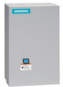
Non-reversing motor starter Size 2 Three phase full voltage Amb compensate bimetal OLrelay Contactor amp rating 45Amp 24VAC 50-60HZ coil Non-combination type Enclosure NEMA type 1 Indoor general purpose use Extra-wide enclosure
