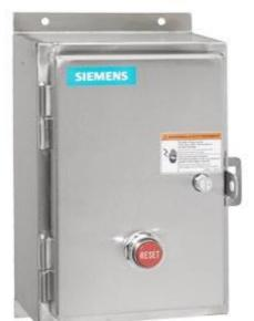
Non-reversing motor starter Size 2 Three phase full voltage Amb compensate bimetal OLrelay Contactor amp rating 45Amp Non-combination type Encl NEMA type 4X 304 S-steel Water/dust tight non-corrosive Extra-wide enclosure
