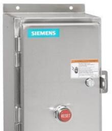
Non-reversing motor starter Size 2 Three phase full voltage Amb compensate bimetal OLrelay Contactor amp rating 45Amp Non-combination type Encl NEMA type 4X 304 S-steel Water/dust tight non-corrosive Extra-wide enclosure
