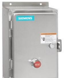
Non-reversing motor starter Size 2 Three phase full voltage Amb compensate bimetal OLrelay Contactor amp rating 45Amp 110VAC 50HZ / 120VAC 60HZ coil Non-combination type Encl NEMA type 4X 304 S-steel Water/dust tight non-corrosive Extra-wide enclosure
