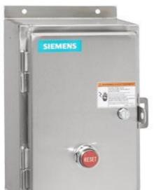
Non-reversing motor starter Size 2 Three phase full voltage Amb compensate bimetal OLrelay Contactor amp rating 45Amp Non-combination type Encl NEMA type 4X 304 S-steel Water/dust tight non-corrosive Extra-wide enclosure
