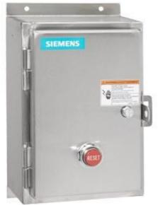
Non-reversing motor starter Size 2 Three phase full voltage Amb compensate bimetal OLrelay Contactor amp rating 45Amp 24VAC 50-60HZ coil Non-combination type Encl NEMA type 4X 304 S-steel Water/dust tight non-corrosive Extra-wide enclosure
