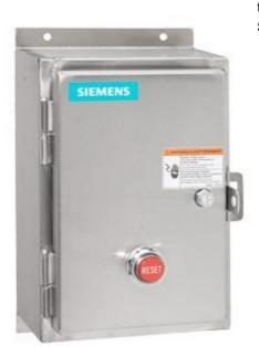
Non-reversing motor starter Size 2 Three phase full voltage Solidstate overload relay OLRelay amp range 13-52a Non-combination type Encl NEMA type 4X 316 S-steel Water/dust tight non-corrosive Standard width enclosure
