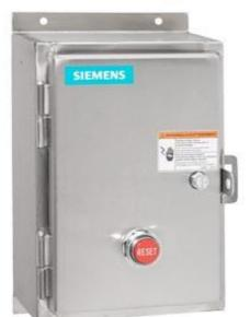
Non-reversing motor starter Size 2 Three phase full voltage Solidstate overload relay OLRelay amp range 13-52a 208VAC 60HZ coil Non-combination type Encl NEMA type 4X 316 S-steel Water/dust tight non-corrosive Standard width enclosure
