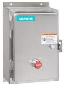
Non-reversing motor starter Size 2 Three phase full voltage Solidstate overload relay OLRelay amp range 13-52a 110VAC 50HZ / 120VAC 60HZ coil Non-combination type Encl NEMA type 4X 316 Ssteel Water/dust tight non-corrosive Standard width enclosure
