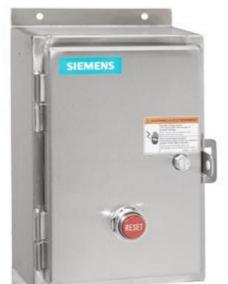
Non-reversing motor starter Size 2 1/2 Three phase full voltage Amb compensate bimetal OLrelay Contactor amp rating 60Amp 208VAC 60HZ coil Non-combination type Encl NEMA type 4X 304 S-steel Water/dust tight non-corrosive Extra-wide enclosure
