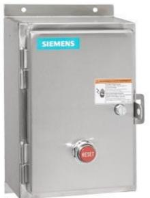
Non-reversing motor starter Size 2 1/2 Three phase full voltage Amb compensate bimetal OLrelay Contactor amp rating 60Amp 110VAC 50HZ / 120VAC 60HZ coil Non-combination type Encl NEMA type 4X 304 S-steel Water/dust tight non-corrosive Extra-wide enclosure
