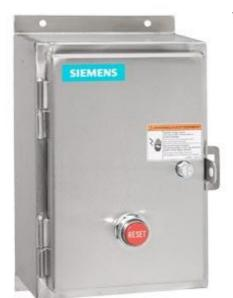
Non-reversing motor starter Size 2 1/2 Three phase full voltage Solid-state overload relay OLRelay amp range 25-100A 24Vdc coil Non-combination type Encl NEMA type 4X 304 S-steel Water/dust tight non-corrosive Standard width enclosure
