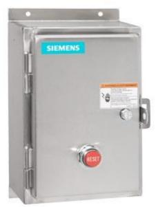
Non-reversing motor starter Size 2 1/2 Three phase full voltage Solid-state overload relay OLRelay amp range 25-100A 208VAC 60HZ coil Non-combination type Encl NEMA type 4X 316 S-steel Water/dust tight non-corrosive Standard width enclosure
