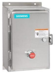
Non-reversing motor starter, Size 2 1/2, Three phase full voltage, Solid-state overload relay, OLRelay amp range 25-100A, 110V 50HZ / 120V 60HZ coil, Non-combination type, Enclosure type 4X 304 S-steel, Water/dust tight noncorrosive, Standard width enclosure
