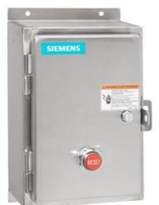
Non-reversing motor starter Size 2 1/2 Three phase full voltage Solid-state overload relay OLRelay amp range 25-100A 24Vdc coil Non-combination type Encl NEMA type 4X 304 S-steel Water/dust tight non-corrosive Extra-wide enclosure
