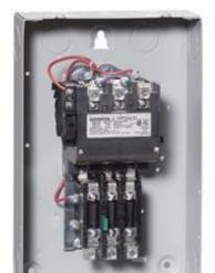
Non-reversing motor starter, Size 3, Three phase full voltage, Amb compensate bimetal OLrelay Contactor amp rating 90Amp 240V 50HZ / 277V 60HZ coil, Non-combination type, Enclosure type 1, Indoor general purpose use
