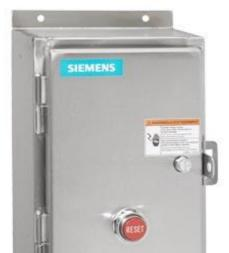
Non-reversing motor starter, Size 3, Three phase full voltage, Amb compensate bimetal OLrelay Contactor amp rating 90Amp 208VAC 60HZ coil, Non-combination type, Enclosure type 4X 304 S-steel, Water/dust tight noncorrosive
